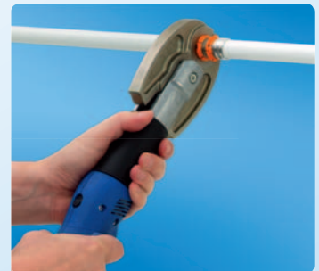
3. Push the pipe into the fitting until the white colour of the pipe is visible in the small window - Press the connection with the tool
